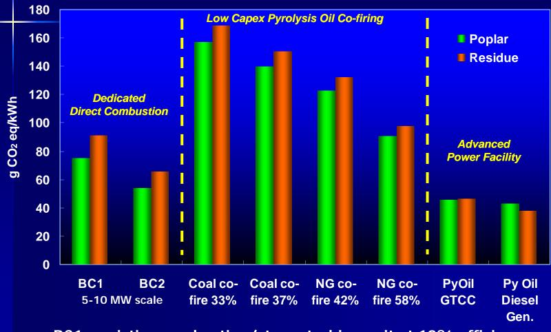
BC1= existing combustion/steam turbine unit at 18% efficiency BC2= modern combustion/steam turbine at 25% efficiency
